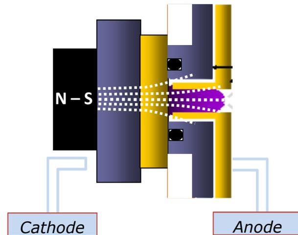
Magnetic field perpendicular to the sample surface
