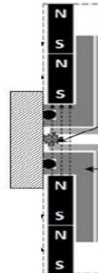
**Magnetic field parallel to the sample surface**
