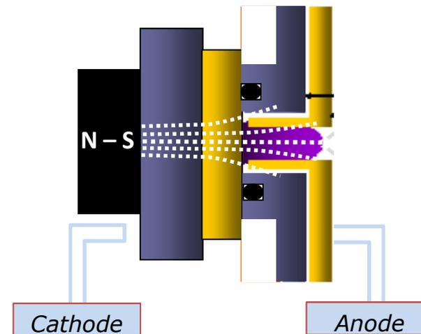
Magnetic field perpendicular to the sample surface
