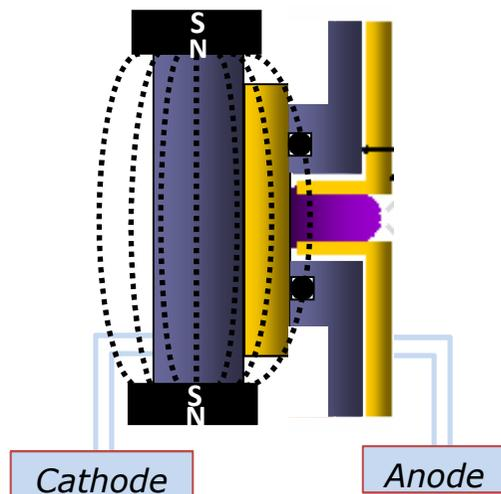
**Magnetic field parallel to the sample surface**
