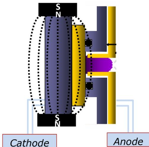
Magnetic field parallel to the sample surface
