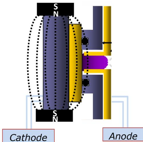
Magnetic field parallel to the sample surface
