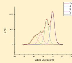
FIG.3- XPS spectrum of Sb 4d3/2 and Sb 4d5/2 on GaSb native wafer. Composition : 71.1% Sb in GaSb and 28.8% Sb in Sb oxide
