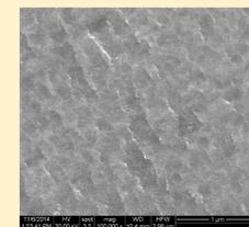
FIG.4- SEM image of GaSb chemical etched surface
