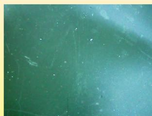
FIG.8 Optical image of AuGeNi/ GaSb surface after ion beam etching
