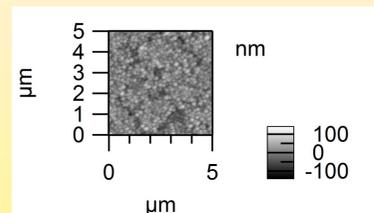
FIG.9 AFM aspect of AuGeNi/GaSb after Ar ion beam etching
