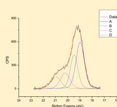
FIG.2- XPS spectrum of Ga 3d lines on native oxides. Composition : 71.5 % Ga in GaSb and 28.5% Ga in Ga oxide
