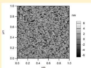
FIG.1- Initial surface aspect of GaSb as a conglomerate of Ga and Sb oxides defining a surface roughness of 1.854 nm
