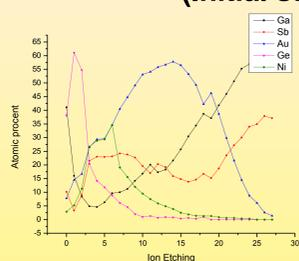
FIG.7 Depth profiling of Au/Ge/Ni in the 28 ion beam etchings controlled by XPS analysis
