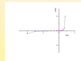
FIG.10 I-V characteristics of MBE Ni/GaSb Schottky diode (Ni thickness ~ 2 nm). This sample had a AuGeNi ohmic contact
