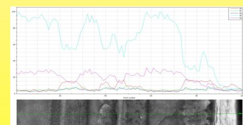
FIG.13 SEM image and elemental distribution on AuGeNi / GaSb interface
