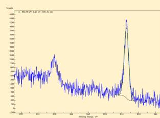
FIG.6 XPS spectra of Au, Ge Ni lines after 16-th ion beam etching
