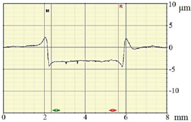
Figure 1 – Profile GD crater, obtained on the sample №1 with protective coating TiN. GD Phofiler-2 parameters are pressure 650 Pa and power 40 W.
