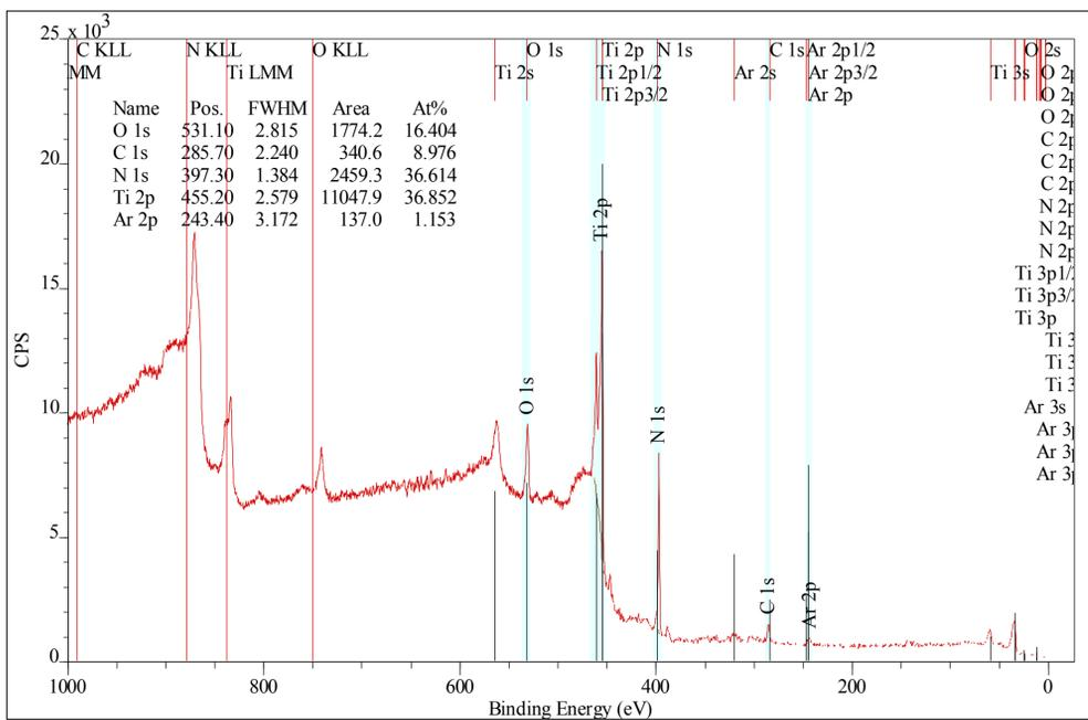
Figure 3—XPS spectra of the sample №1 with protective coating TiN and atom concentration, obtained in program CasaXPS.
