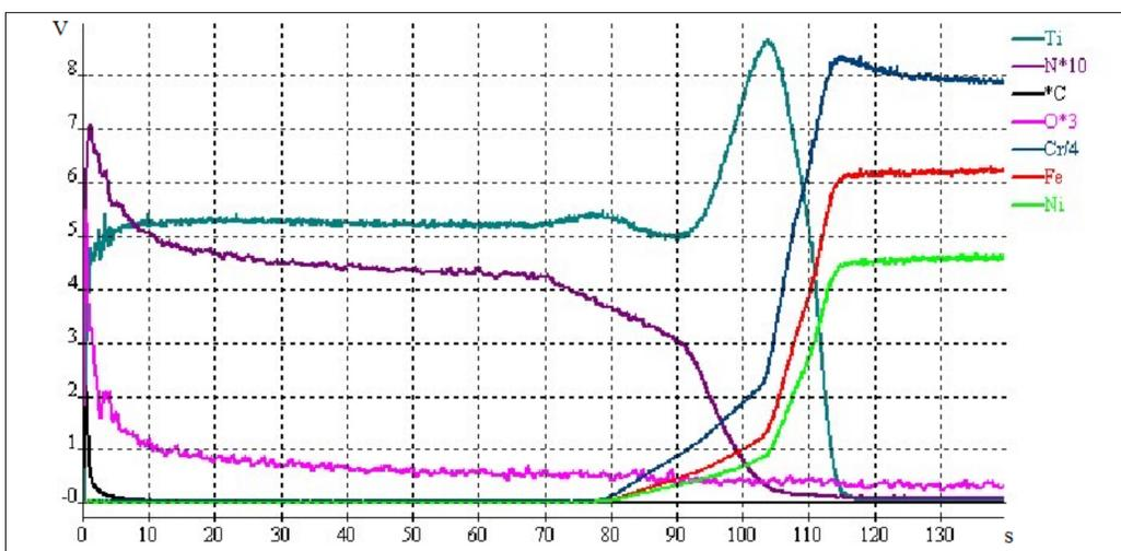
Figure 4 – Depth profile signals High Dynamic Detectors of the sample №1 with protective coating TiN.
