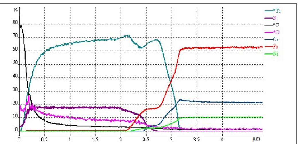
Figure 5 – Quantitative depth profile of the sample №1 with protective coating TiN.
