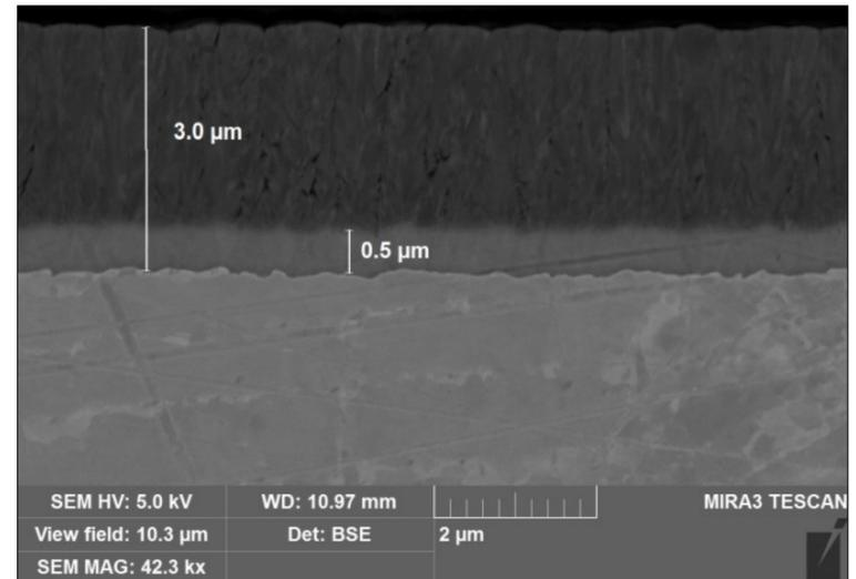
Figure 2 – SEM image sample №1 with protective coating TiN.
